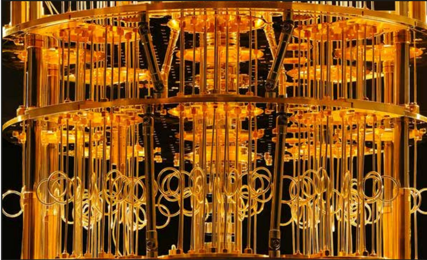
Dilution refrigerator of an IBM Q quantum computer
