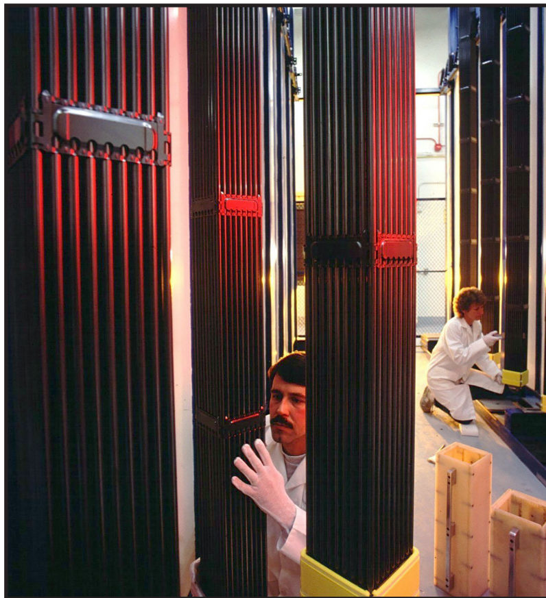
Nuclear fuel assemblies under inspection
